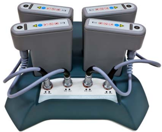
Figure 3: Charging unit with four batteries (front panel view)
